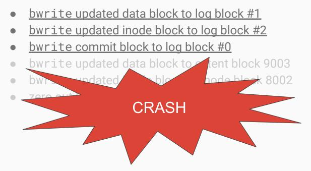
On recovery, we inspect the log and find that the committed flag in log block 0 is set to 1. Thus we have the entire operation in the log, so we can replay the operations, updating the data and inode blocks, and then clear the log.
